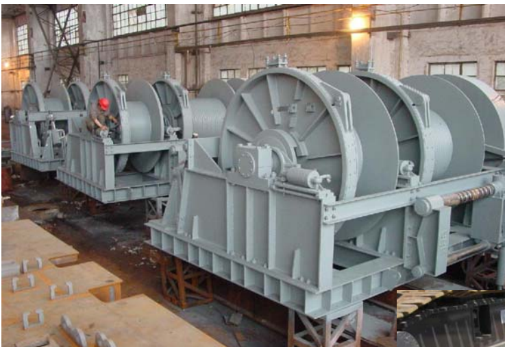
Model : DDE-80T-FC-S-R - Electric Driven - Frequency Control - Double Drum with Spooling Device
