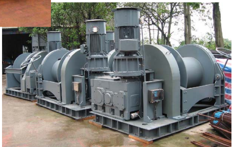
Model : DE-36T-36X500M-FC - Pull Load 36 Tons - with Frequency Control
